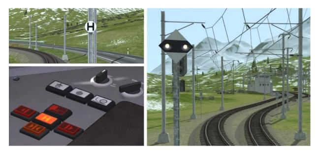
The signal shown above right is provided at the approach to request only stations. It is activated by passengers at the station by pressing a button at the information point. When activated the two white lights on the signal board flash together to indicate to the driver that passengers wish to board their train.
