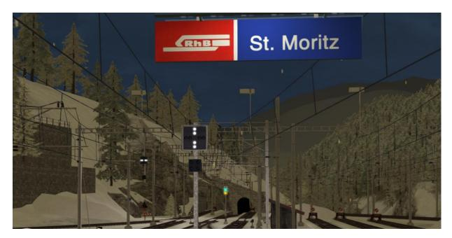
At St. Moritz there are only two main departure signals, one that applies to Bernina Line departures and a second for all departures in the direction of Samedan. If the main departure signal applies to a specific platform then the associated Clear Track Signal displays four vertical white lights. If the main departure signal does not apply to a platform then the associated Clear Track Signal displays four horizontal white lights and the driver must not pass the indicator.
