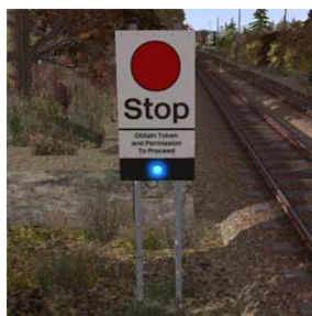
Direction Stop Board (DSB) with TPWS Status Indicator Lamp
